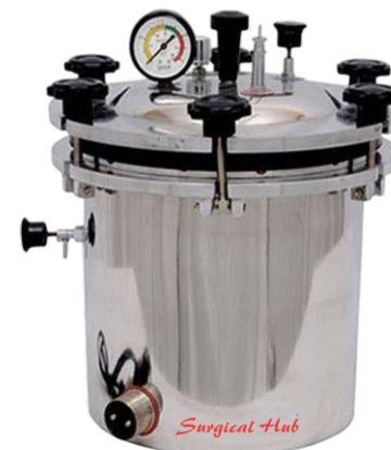
DNS - 412 AUTOCLAVE (PORTABLE) SINGLE/DOUBLE DRUM ALUMINUM Seamless construction made of aluminium alloy with turning on lid highly polished. It comes with one stop cock (continues bleeding valve), safety valve and pressure guage. Size: 12"x12", 12"x14", 12"x20" Note : Also Available in S.S. Model
